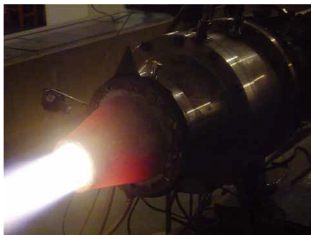
1600°C gas wind tunnel coating scouring environment
