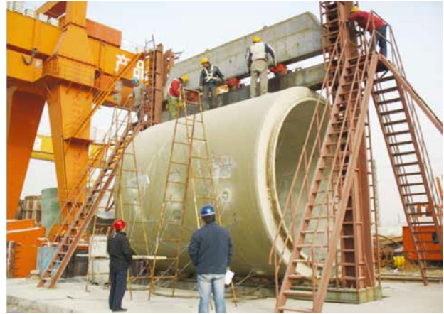
Prototype diagnosis test of complex hydraulic concrete PCCP service behavior
