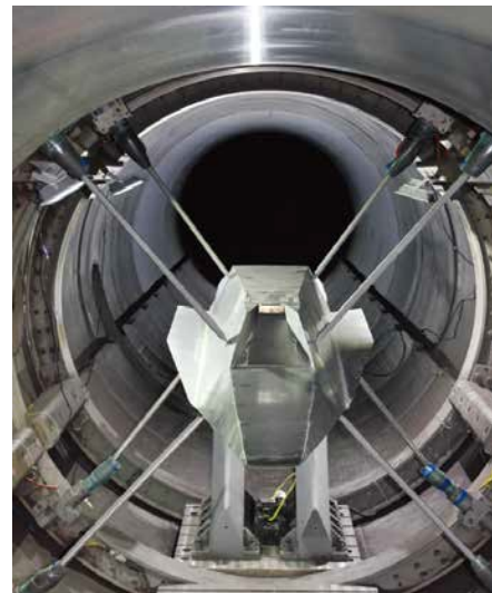
The world's first integrated experiment on a powered aircraft in reproduced hypersonic flight conditions
