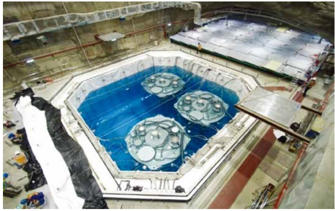
Top view of the remote experimental hall, 3 neutrino detectors are placed in the water Cherenkov detector pool and the resistive plate detectors are visible at the far end
